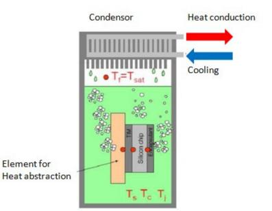
Fig. 4-1. Evaporation cooling of a silicon chip ©3M.
