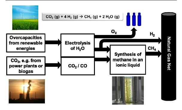
Fig. 2-3. Using the Sabatier-process to store energy inside the natural gas net.
