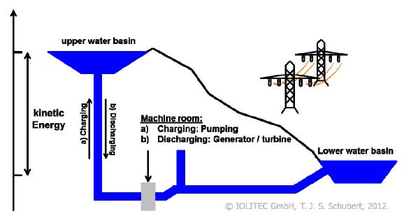
Fig. 2-1. Principle of a Pump storage.
