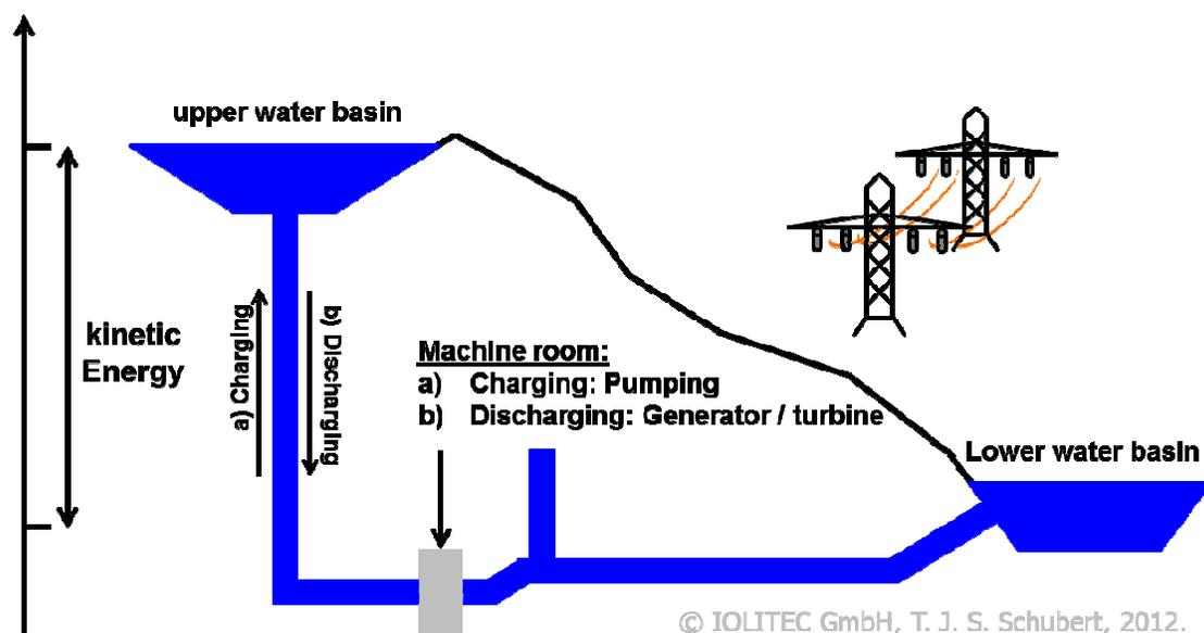
**Fig. 2-1.** Principle of a Pump storage.
