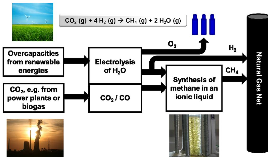
**Fig. 2-3.** Using the Sabatier-process to store energy inside the natural gas net.
