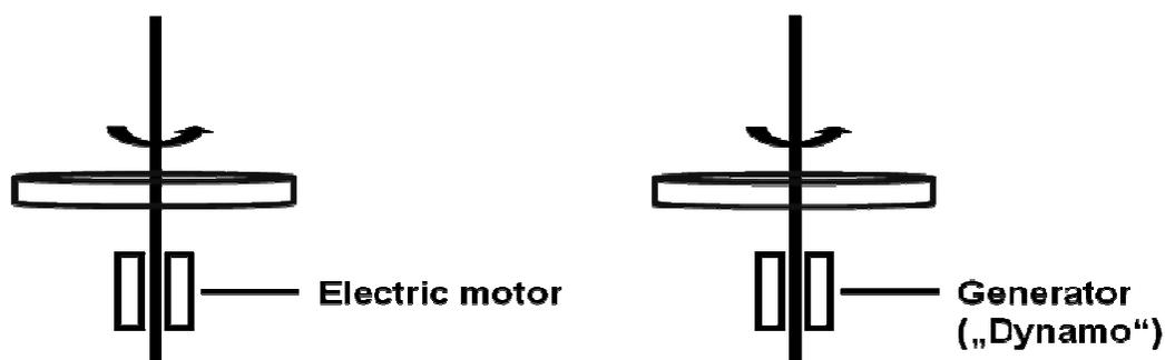
**Fig. 2-4.** Charging (left) and discharging (right) of the balance wheel.
